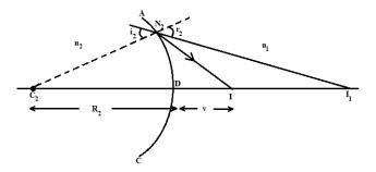
Using the relation refraction at spherical surface,  $\frac{-n_2}{DI_1} + \frac{n_1}{DI} = \frac{n_2 - n_I}{DC_2}$ .....(2)
