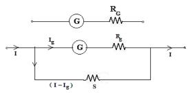
Let S be the shunt resistance to be connected to convert it into an ammeter of range 0 to I. The value of S should be such that, when a current I enter the instrument, only a small portion  $I_g$  flows through galvanometer.
