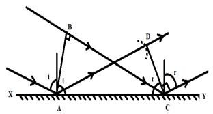
In order to construct the reflected wavefront, we draw an arc at D of radius vt with A as centre. The tangent from C touches this arc at D. Hence CD is the reflected wavefront and let r be the angle of reflection.
