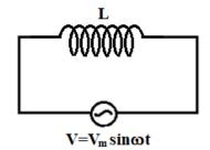
Let the source supplies a sinusoidal AC voltage to inductor & is given by
