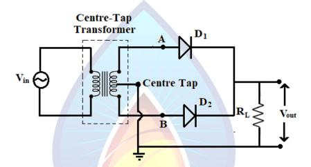
The circuit diagram is as shown in the figure. The diodes  $D_1$  and  $D_2$  with a load resistor  $R_L$  are connected across the secondary of the transformer. The  $R_L$  is connected to the center tap of the secondary transformer. The A.C voltage to be rectified is applied to the primary of the transformer.
