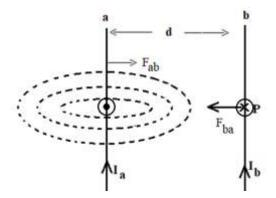
The magnitude of the magnetic field at any point P on the conductor 'b', due to current  $I_a$  in the conductor 'a' is;
